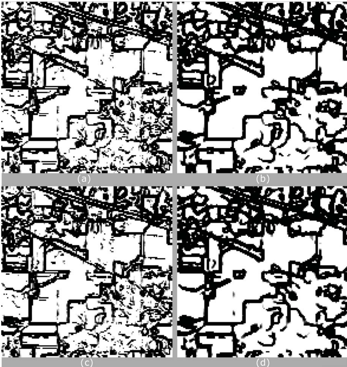
Figure 5.5.3: Comparison of the effect of the structure tensor using the time evolution after iterations n of the \lambda -entry of the diffusion tensor of TAND-EED applied to Indian Pines image. \sigma = 0.8 , \tau = 2 , \psi = \mu'_1 's 55 th percentile. (a) \lambda using the classical structure tensor, n = 1 . (b) \lambda using the classical structure tensor, n = 4 . (c) and (d) same as (a) and (b) using the heat weighted structure tensor.
