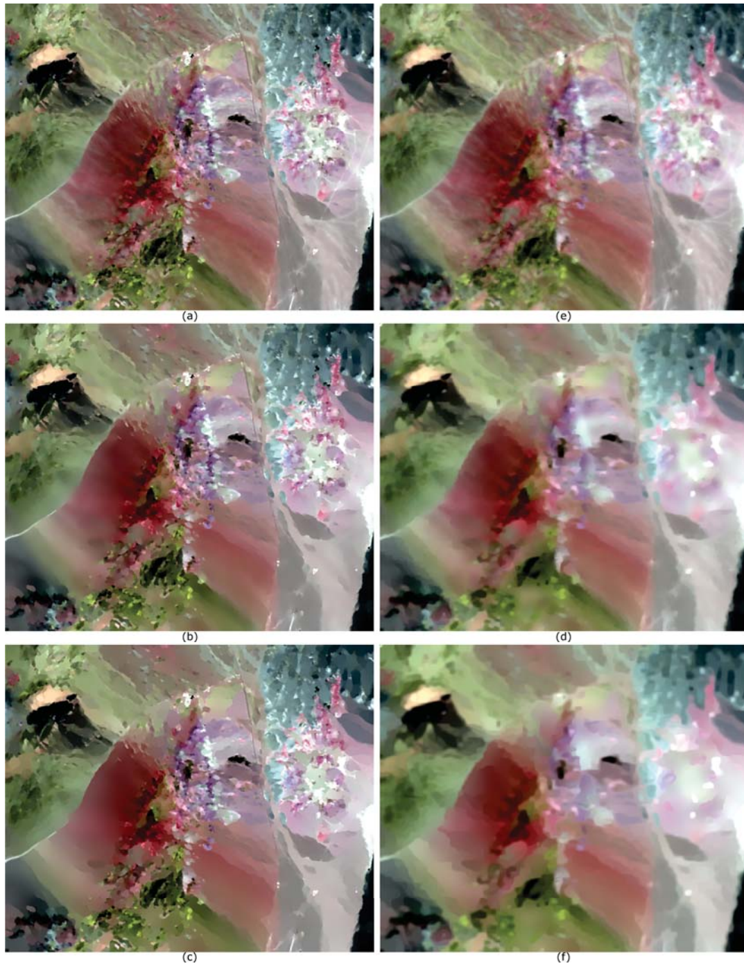
Figure 5.6.2: Comparison of the proposed TAND-EED with Weickert's TAND-EED applied to Cuprite image. (a) n = 1 using the proposed TAND; (b) n = 5 using the the proposed TAND-EED; (c) n = 15 using the proposed TAND; (d), (e), and (f) are the same as (a), (b), and (c) respectively but using the Weickert's TAND.
