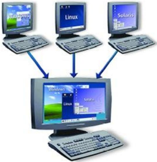
In computing, a **virtual machine (VM)** is an emulation of a particular computer system.
