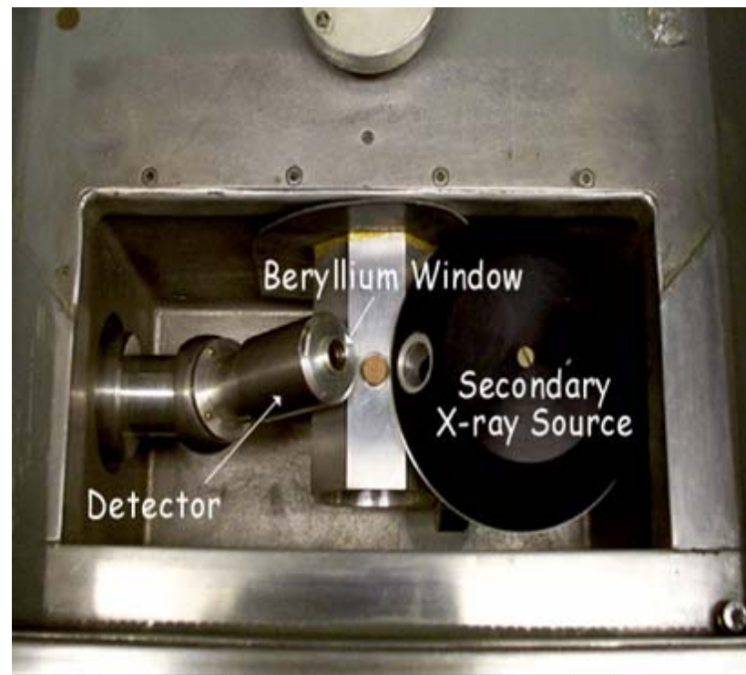
Figure 6(b): The XRF sample chamber with Si (Li) detector
