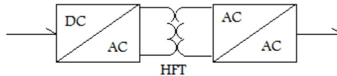
Figure 5.15 Multi-Stage Inverter with HF Transformer in AC Converter
