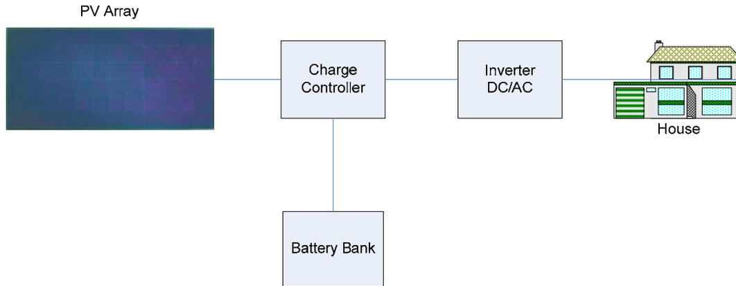
Figure 5.1 Stand-Alone Photovoltaic System
