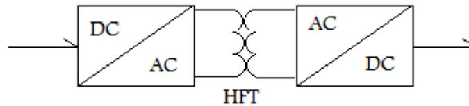
Figure 5.16 Multi-Stage Inverter with HF Transformer in DC Converter
