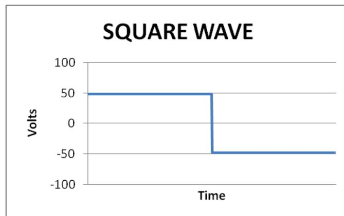
Figure 5.9- Example Voltage Square Wave
