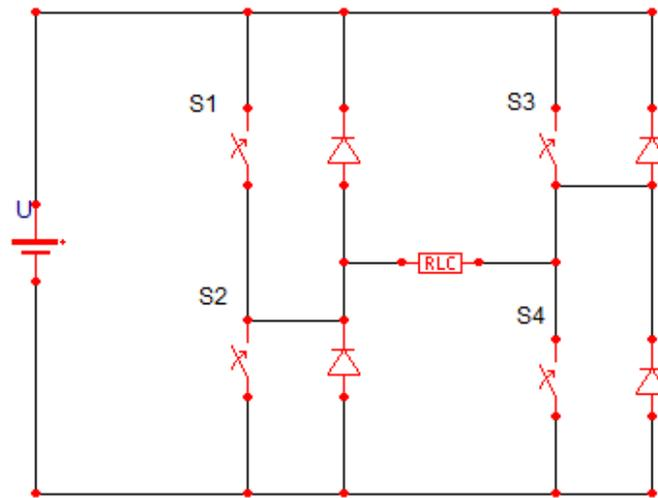
Figure 5.8-Single Phase Inverter Conceptual Circuit
