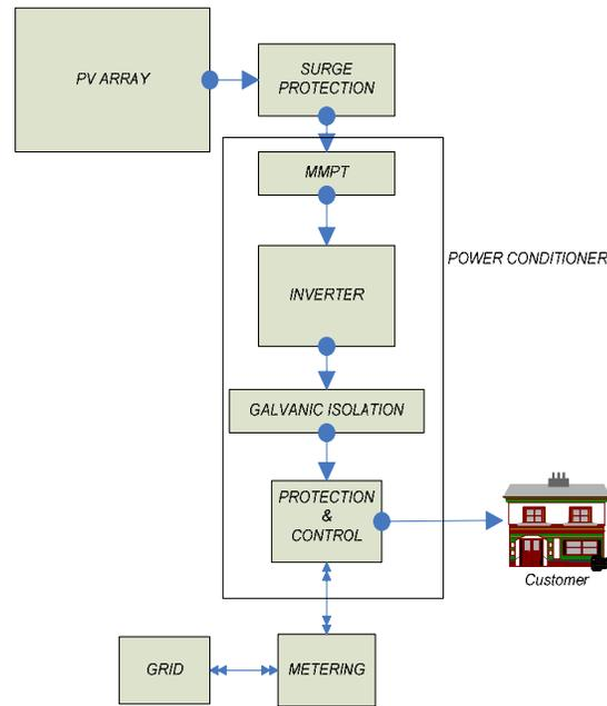
Figure 5.10-Grid-Connected PV System Block Diagram
