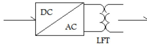
Figure 5.14 Single-Stage Inverter with LF Transformer
