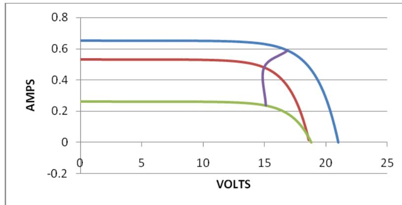
Figure 5.11- I-V Curves for a PV Module at different operating conditions
