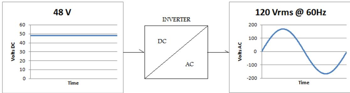
Figure 5.7 Representation of DC to AC conversion Process
