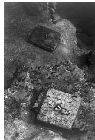
Fig. 2 Photograph of settlement plate attached to a base plate 3 months after deployment
