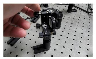
**6. De-activate** the necessary mirrors by flipping their kinematic mount horizontally (parallel to the table).
