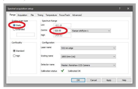
**11. Choose** the Edge filter placing previously from Configuration  $\rightarrow$  Laser name.
