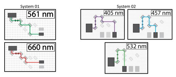
The optical setups utilize a fused silica ( $SiO_2$ ) broadband dielectric 400-750 nm mirror placed on a kinematic mirror mount with 3 adjusters. All mirrors are fixed in position with an optical post, post holder, and a swivel base adapter. However, some mirrors contain, in addition, a flip mount adapter. The flip mount adapter allows the user to either place the mirror upwards and reflect the incoming light source or downwards so that the source continues towards the next mirror.
