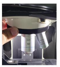
23. Set optical magnification on the WiRE software.
