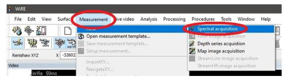
**10. Change** the Grating scan type to "Static" mode from the "Range" tab in the "Spectral acquisition setup" window.
