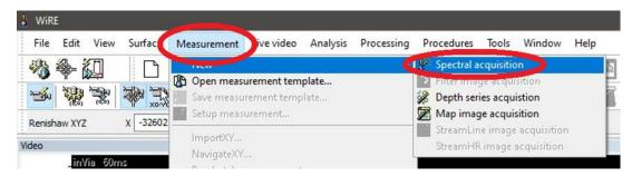
**6. Place** "Extended" mode from the "Range" tab and the "Spectral acquisition Setup" window with the desired spectrum range.
