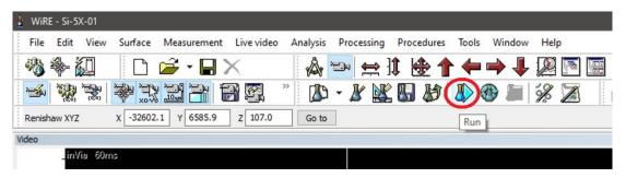
**24. [OPTIONAL] Run** again in "Extended" mode from 100 to 1000 cm<sup>-1</sup> to validate offset.
