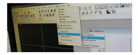
**22. Place** value to fix offset (positive values are subtracted and negative values are added) and click "OK".
