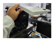
**8. Verify** that the correct edge filter is placed (varies per laser excitation line).
