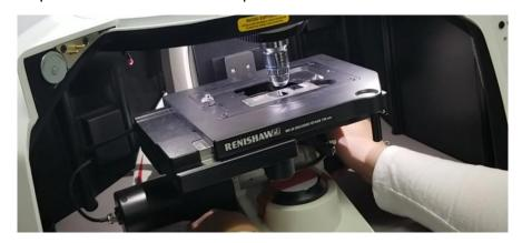
**3. Move** sample until the light is placed between the corner of the plate and sample. **Move** montage vertically to observe a gradient between corner of the plate and sample.
