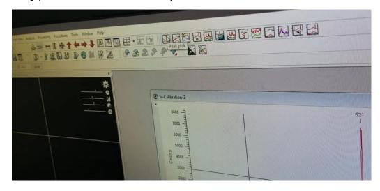
**21. Fix** peak shift from Tools  $\rightarrow$  Calibration  $\rightarrow$  Offset.
