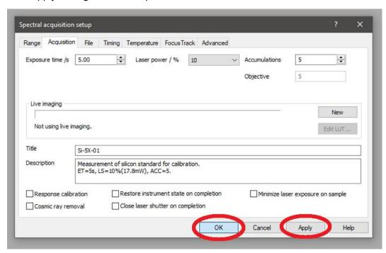
**8.** Adjust laser power, exposure time, and accumulations.
