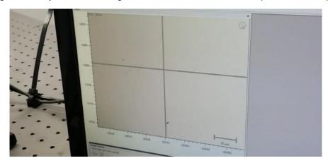
**4. Focus** until the line between the plate and sample is seen.
