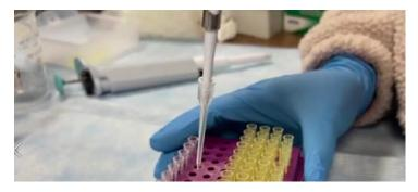
4. Press top button on micropipette two times and hold.
