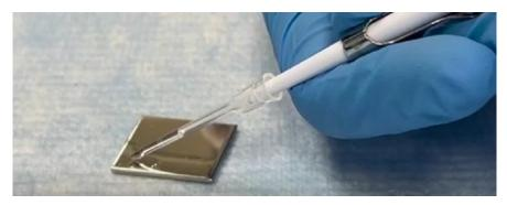
8. Release solution slowly moving to the upper righthand side of the substrate.
