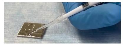
**11. Release** solution slowly moving downward on the lefthand side of the substrate.
