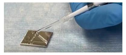
**10. Release** solution slowly moving to the upper lefthand side of the substrate.
