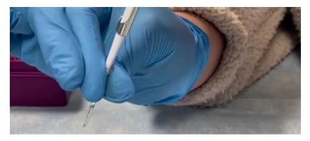
14. Press micropipette lower micropipette button to release the micropipette tip.
