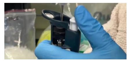
**15.** Place micropipette tip on a crystalline dish for unwanted material.
