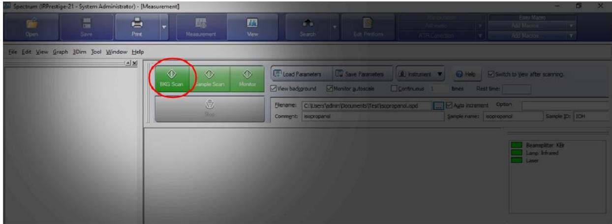
The interface will change from “Measurement” to “View” when the spectra is acquired.
