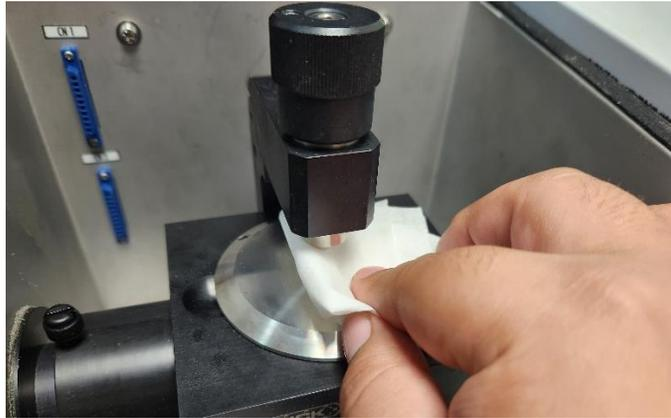
2. **Place** sample in ATR plate and adjust tip.
