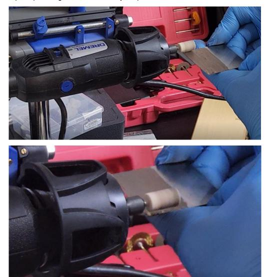
**9. Slide** the aluminum substrate on the polishing point uniformly with enough force to feel the point polishing the substrate. **Repeat** process for 5-10 minutes.
