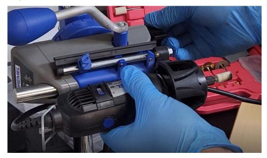
8. Turn on the DREMEL 200-1/21 drill to the low option (15,000 RPM).
