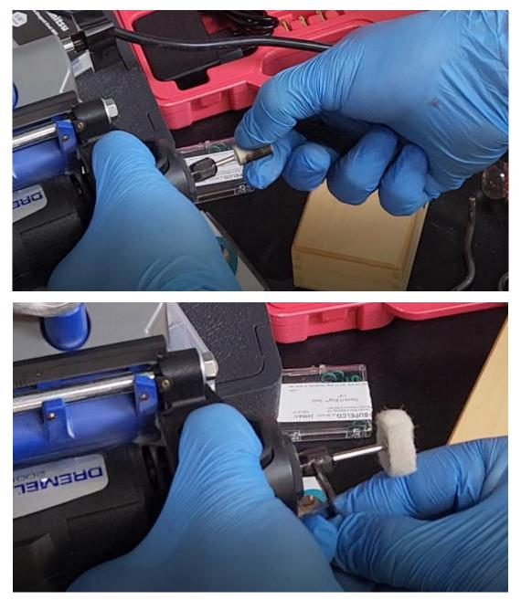
**11. Polish** substrate by wiping uniformly for 5 to 10 minutes.
