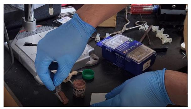
2. Swipe back and forth the polishing compound on the material until all the substrate surface is covered.
