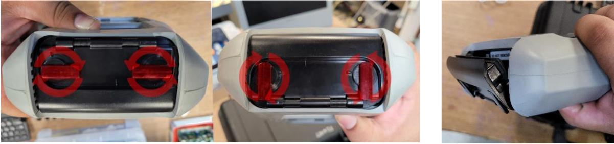
4. **Insert** SD memory inside the portable Raman spectrometer.
