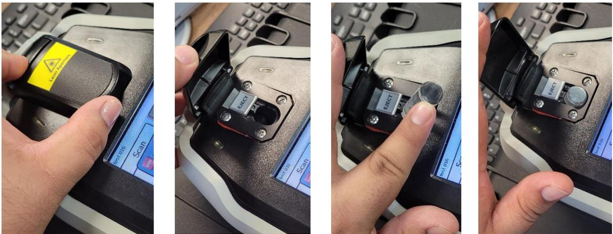
4. Press "ARM" button to indicate that the Raman contains a sample.
