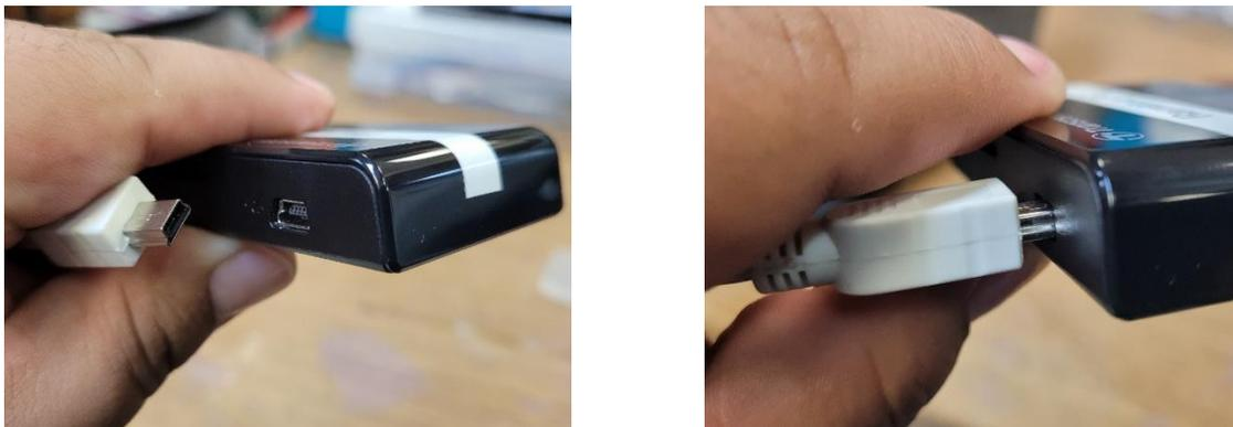
4. **Connect** the USB to microSD adapter cable to the computer to transfer files.
