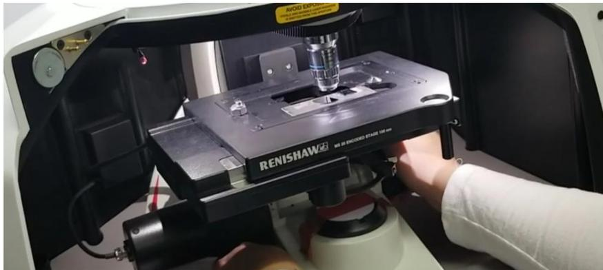
3. **Move** sample until the light is placed between the corner of the plate and sample. **Move** montage vertically to observe a gradient between corner of the plate and sample.
