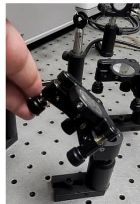
6. **De-activate** the necessary mirrors by flipping their kinematic mount horizontally (parallel to the table).
