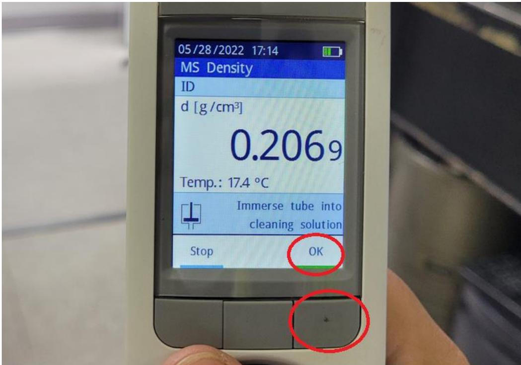
8. **Insert** plastic tube in the waste beaker to remove water inside the density meter.
