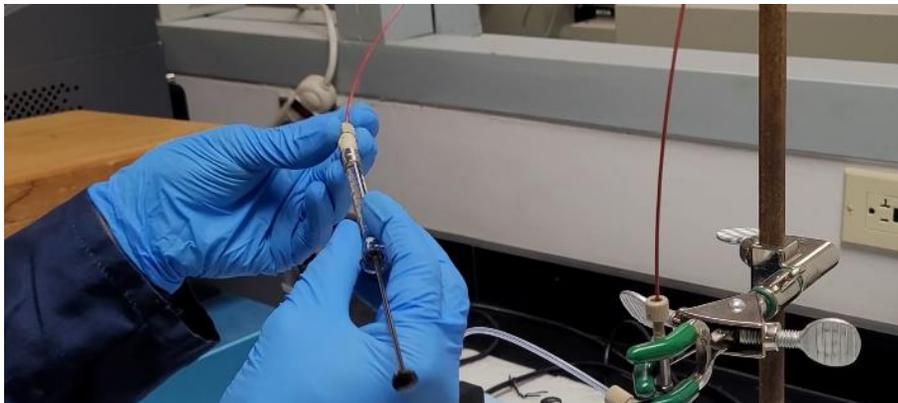
8. **Rinse** tubing with 250  $\mu\text{L}$  of ethanol.
