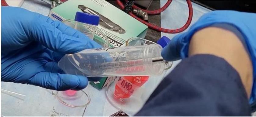
5. **Clean** infusion tubing with ethanol using Pasteur pipette.
