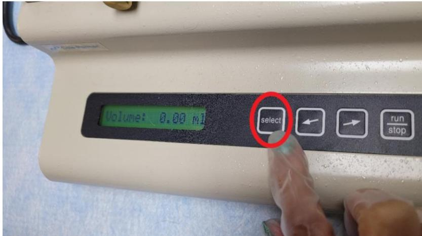
15. Set flow rate to  $500 \frac{\mu L}{hr}$  (default) by pressing the SELECT button on select flow rate.
