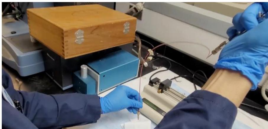
9. **Place** syringe with ethanol on infusion pump and deposit ethanol on a Kim wipe to clean the ESI needle.
