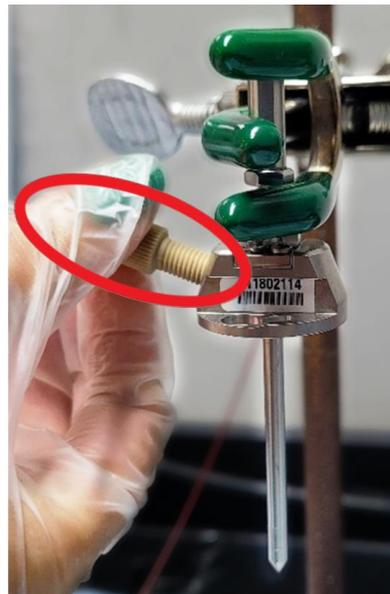
5. **Connect** PEEK infusion tubing through the PEEK super flangeless nut to the ESI needle port. Hand tight the flangeless nut.
