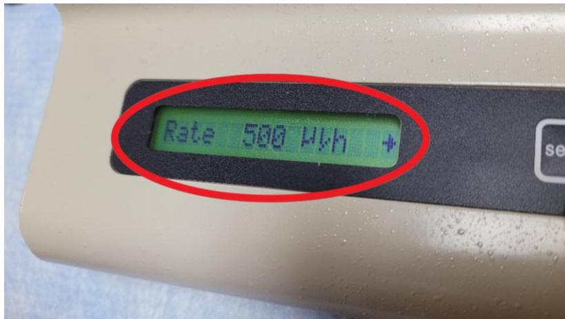
Adjust flow rate depending on the substrate surface.
