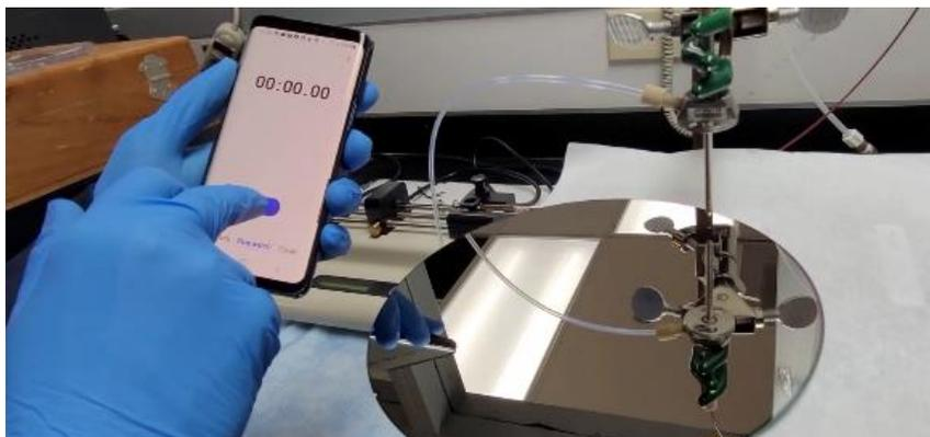
11. **Stop** deposition when completed by simultaneously pressing the RUN/STOP button and closing the valve of the two-stage regulator.
