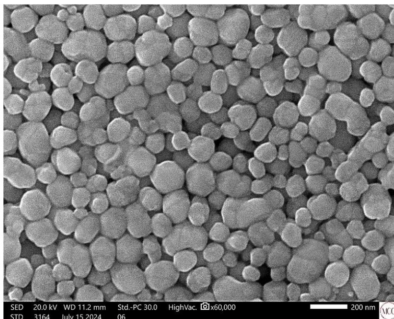
Figure 2. FE-SEM micrographs obtained for AgNPs
