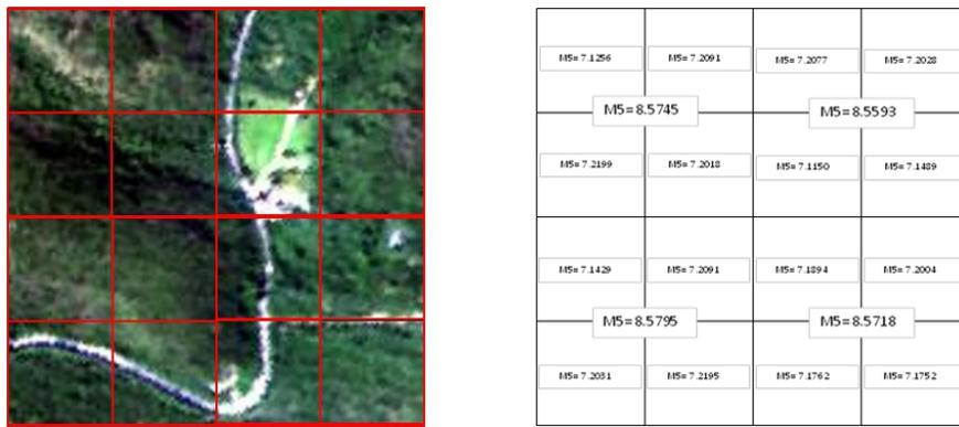
Figure 6-17. Quadtree partitioning using norm of the Shannon Entropy with global index  $M5 = 8.5589$  for Guanica at 4m resolution.
