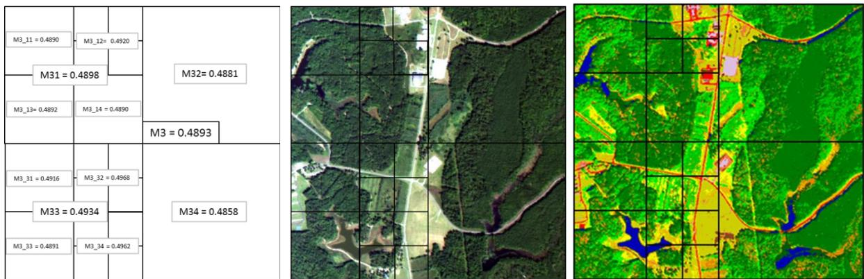
**Figure 4-5. Partitions using the mean of all values in the image with global index M2 = 0.4893.**
