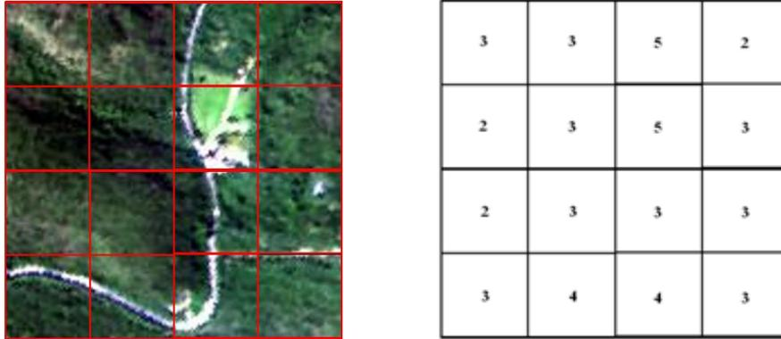
**Figure 6-26. Classes per Partition resulting from the Local unmixing analysis using sacNMF for Guanica at 4m.**
