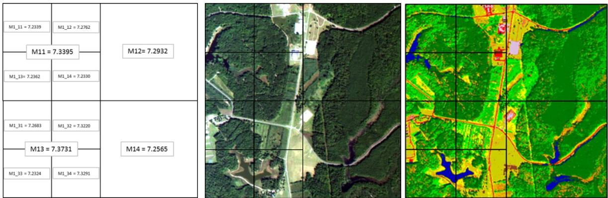
Figure 4-4. Partitions using the mean distance from spectral centroid with global index M1 = 7.3298.
