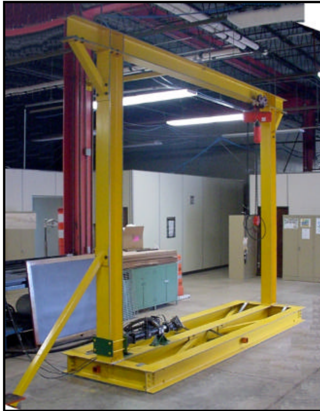
Figure 3.11 Reaction Mass fixed to the Laboratory Strong Floor.
