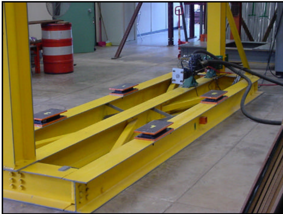
b) Linear Bearing System mounted on Reaction Mass.
