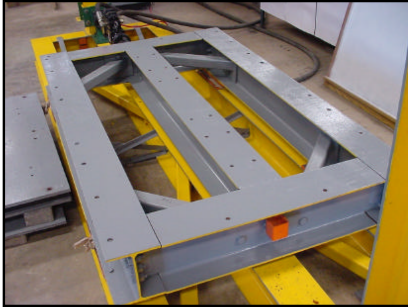
(a) Simulator Platform Welded Steel Frame.
