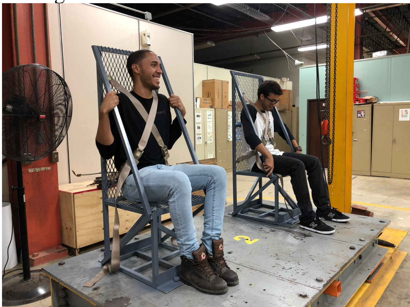
Figure 1. Test Subjects Experiencing Dynamic Loads on the “Seismic Chair”
