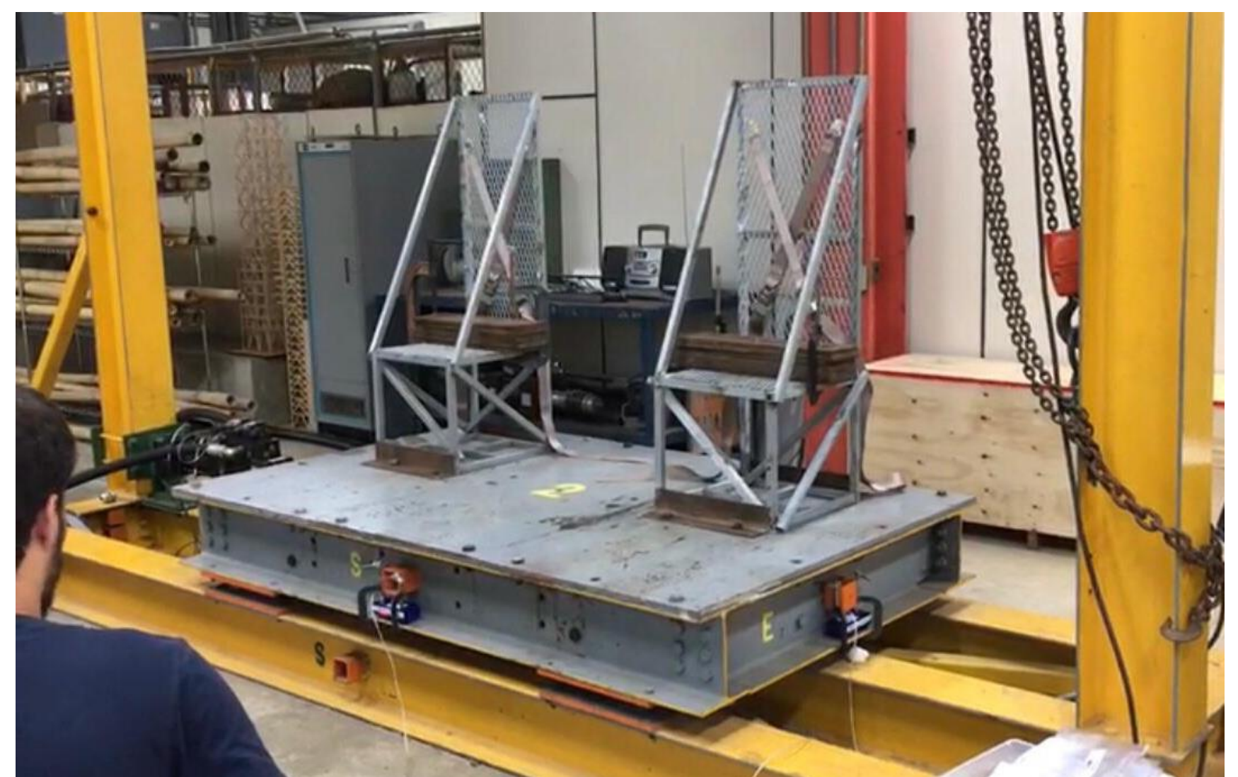
Figure 4. Shake Table Calibration With Chairs and Weight Applied
