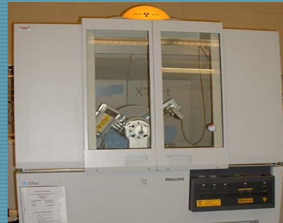
XRD Tin/Polycarbonate/Leaded enclosure
