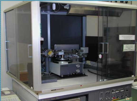
XRD Tin/Polycarbonate/Leaded enclosure
