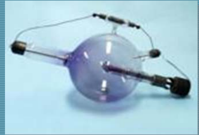
Early X-Ray Tube (1899): This tube is a specimen of the first type of gas x-ray tube to incorporate a water-cooled anode. The hollow anode was supplied with water by gravity feed from a supply held in the side bulb. This type of tube was introduced by Mueller about 1899.
