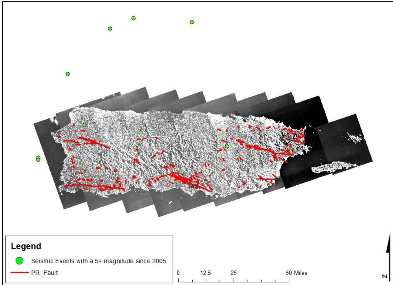
Figure 5. Faults (red lines) and magnitude 5+ earthquake epicenters (green dots) plotted over a SLAR composite from Puerto Rico.
