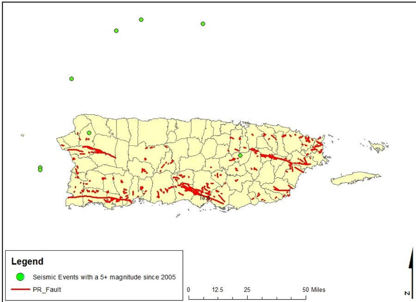
Figure 6. Faults (red lines) and magnitude 5+ earthquake epicenters (green dots) plotted over a municipal map of Puerto Rico.
