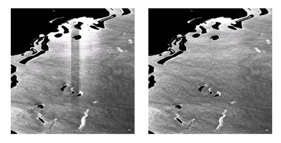
Figure 3: Original subset image with central stripe (left) and after halo suppression (right).
