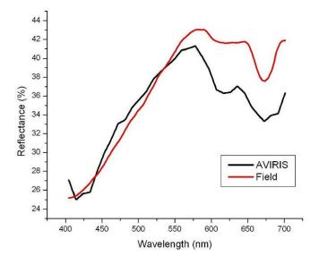
Water column correction validation using a sand target.
