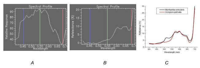
Figure 6: AVIRIS coral spectrum without water column correction (A) and after the correction (B). Representative field spectra from two species of corals is shown for comparison (C).
