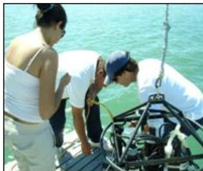
**Figure 4b:** Sampling with the sediment grab.
