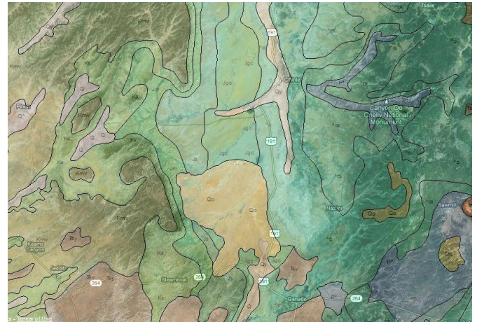
Fig. 3. (Clockwise) An USGS hybrid map for the Chinle formation in Arizona, followed by the same region with a lower transparency and finally the SAM supervised classification created by ENVI 4.8. In SAM image blue marine colors at right indicate correlation with the Chinle Fm. (aqua color) in the USGS maps , while yellow colors tend to indicate the Glen Canyon Group (180-210 Ma) denoted by greener variations in the geological maps.
