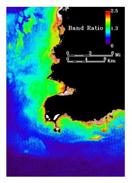
FIG. 8. Sediment Band Ratio (Green/Blue) for coastal waters of Cabo Rojo. Cold colors are more clear water and hot colors are water with more suspended sediment.
