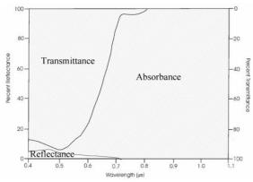
FIG. 1. Spectral curve of clear water. Clear water reflects very little solar irradiance but transmit most of it in the visible spectrum (obtained from Farooq S. 2011).
