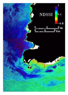
FIG. 7. Normalized Difference Suspended Sediment Index (NDSSI) for coastal waters of Cabo Rojo. Cold colors are more clear water and hot colors are water with more suspended sediment.
