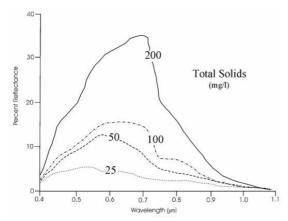
FIG. 2. Spectral curve of water with different concentrations of suspended sediment. The amount of suspended sediment in water is proportional to the reflectance of water (obtained from Farooq S. 2011).
