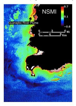
FIG. 6. Normalized Suspended Material Index (NSMI) for coastal waters of Cabo Rojo. Cold colors are more clear water and hot colors are water with more SM.
