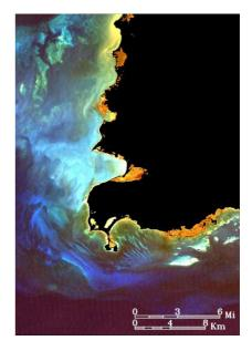
FIG. 5. True Color Image with the mask developed from the K-means image data.
