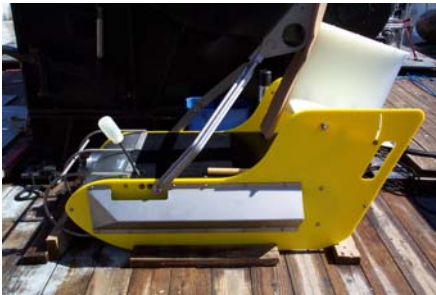
Figure 3. Shown on deck, real-time underway data collection system NuShuttle Undulating Underwater Vehicle carrying CTD_Fluorometer, Fast Repetition Rate Fluorometer (FRRF) and Beam-c (660) transmissometer.
