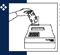
Lift the TD-700's sample chamber door and the unique filter cylinder slips out easily; it is configured to allow four different filter combinations.
