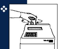
Seat the filter cylinder back in its chamber. With four filter pairs installed, the user can now switch between four different fluorescence analyses in seconds easily, by rotating the cylinder.
