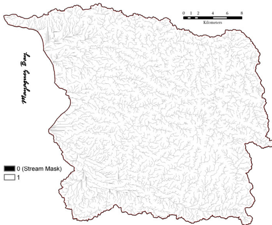
Figure 21. Stream mask layer incorporated in the GIS model in order to exclude erosion estimations corresponding to channels.
