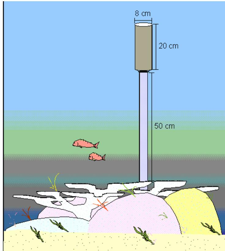
Figure 3 – Sediment trap for field sampling
