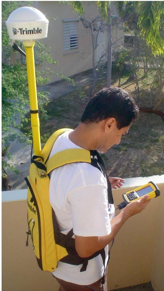
**Figure 11:** GPS backpack instrument to be used to map the shoreline in Arecibo. Image taken from GERS Laboratory website.
