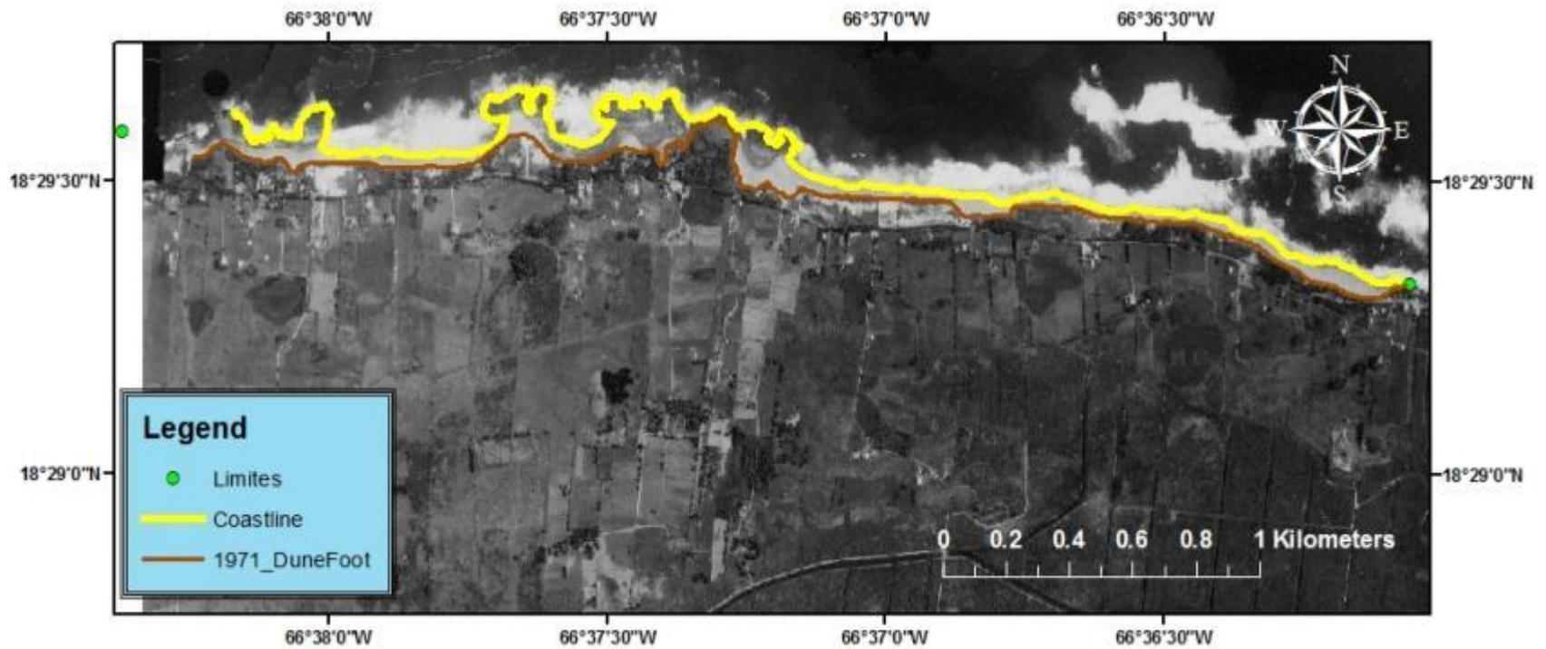
**Figure 6:** Black and white aerial photograph of Barrio Islote, Arcibo, Puerto Rico in 1971. The photo is damaged in the Northwest corner which impede the digitizing of the coastline and dune foot in that end. Aerial photograph provided by the DRNA.
