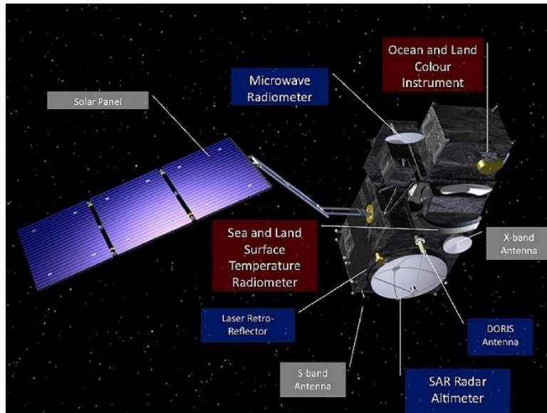
**Figure 4:** Main instruments of the Sentinel-3 mission: Ocean and Land Colour Instrument (OLCI), Sea and Land Surface Temperature Radiometer (SLSTR), SAR Radar Altimeter (SRAL), MicroWave Radiometer (MWR). (Source: Copernicus Sentinel-3, <https://directory.eoportal.org/web/eoportal/satellite-missions/c-missions/copernicus-sentinel-3>)
