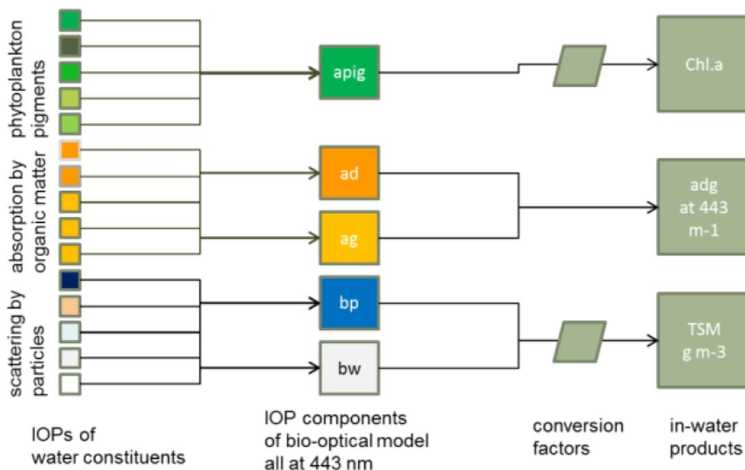
**Figure 7:** Inherent optical properties (IOP) components for bio-optical model (Source:
