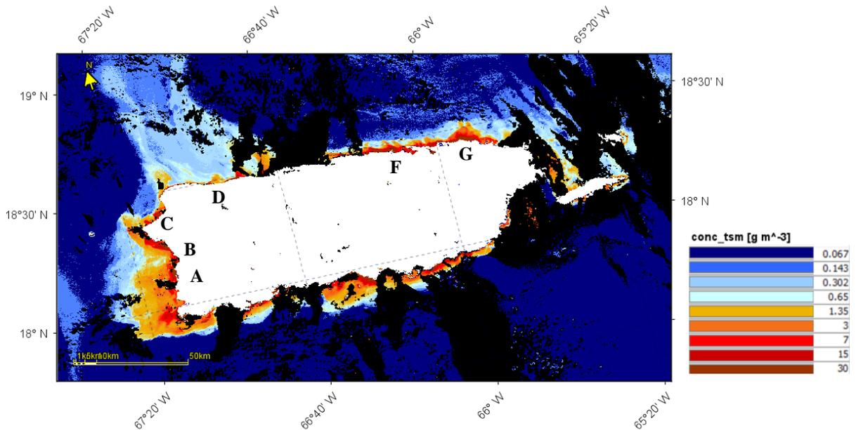
**Figure 11:** Total Suspended Matter (TSM) concentration retrieved from Sentinel-3 OLCI on September 29, 2017. The area in black indicates the clouds present. Discharge from some rivers: (A) *Río Guanajibo*, (B) *Río Grande de Añasco*, (C) *Río de Culebrinas*, (D) *Río Grande de Arecibo*, (F) *Río de la Plata*, (G) *Río Grande de Loíza*.
