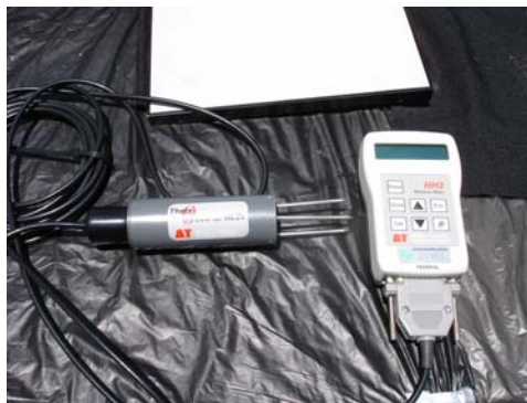
Figure 7: Thetaprobe ML2x moisture sensor
