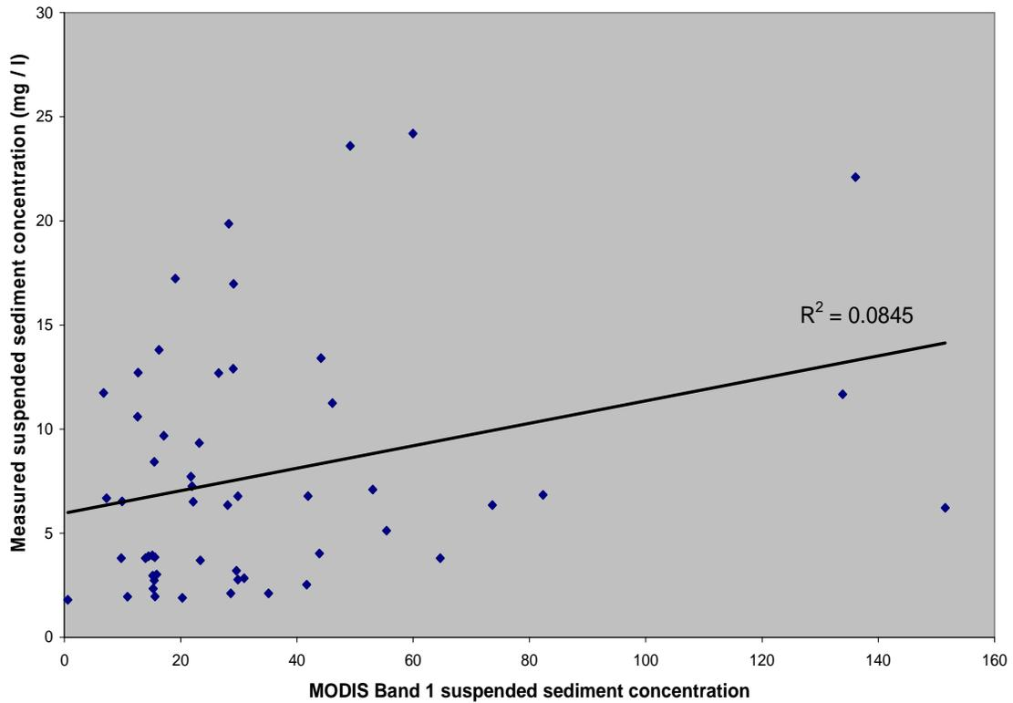
*Figure 7: Relationship of Suspended sediment concentrations between field data and MODIS Terra 250 m Band 1 estimates.*
