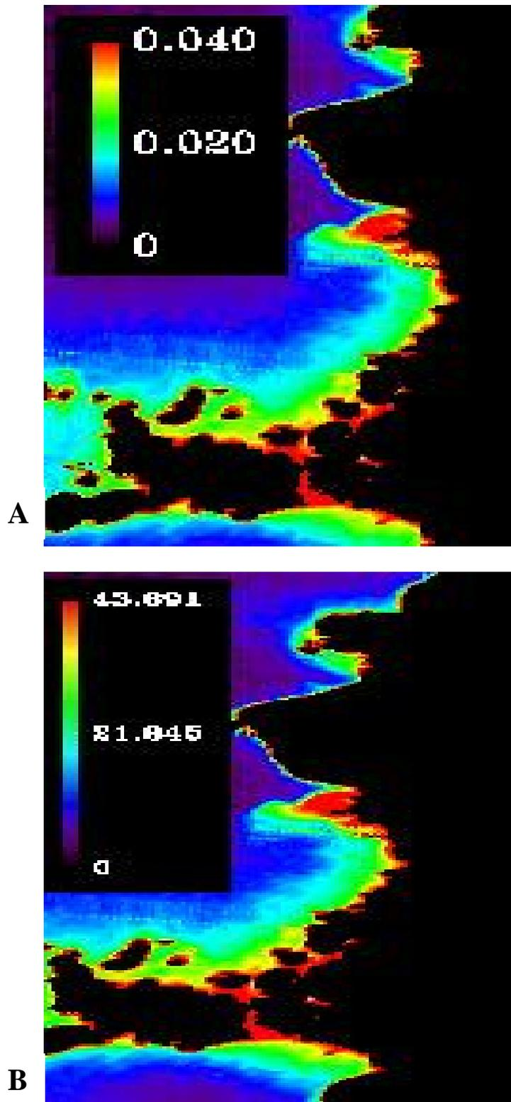
Figure 8: MODIS Terra 250 m Band 1 images from October 4, 2001 generated using ENVI 4.2 (A: Image after atmosphere correction; B: Image after application of algorithm)
