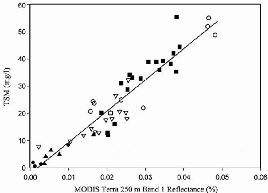
Figure 6: Total suspended matter as a function of atmospherically corrected MODIS Terra 250 m Band 1 reflectance (from Miller and McKee, 2004)
