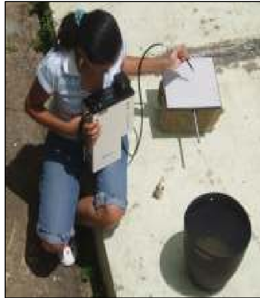
Figure 7: Mixture of 7oz of sediment and water measurement with the HR-1024.
