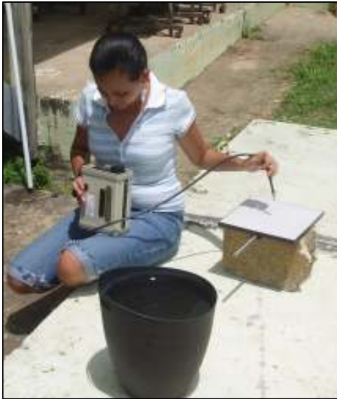
Figure 6: Mixture of 7oz of sediment and water measurement with the GER-1500.
