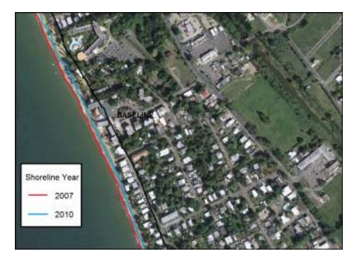
Figure 4: DSAS Final results. Shoreline changes can be seen. GERS Laboratory.
