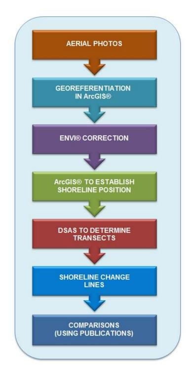
Figure 2: Methodology flow chart. Processes before obtain final results.
