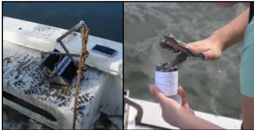
Figure7. Sediments collector (left) and how the sediments were store (right).
