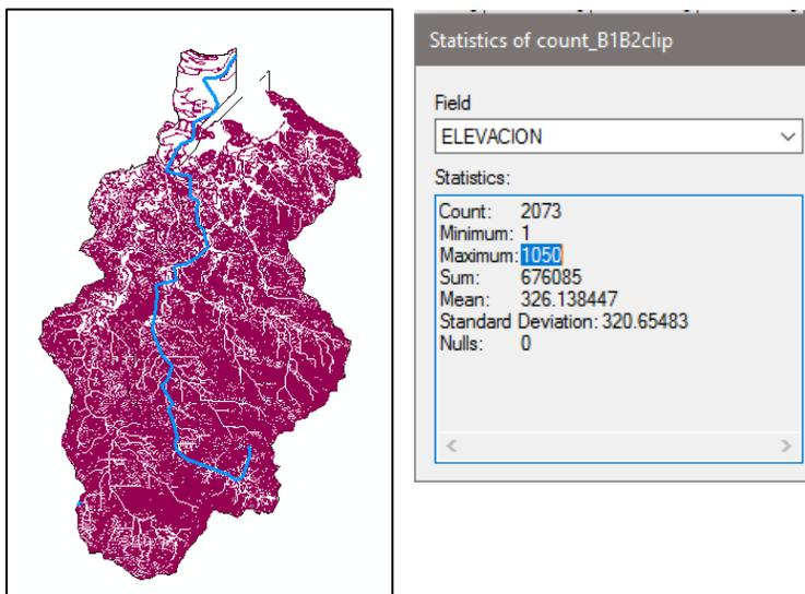
Figure 4. Elevation calculated using the program ArcMap. Lower elevation is 1 m, the highest elevation is 1,050 m, and mean elevation is 326 m. White lines are streams and tributaries, blue line is Río Espiritu Santo, and purple color is the elevation.
