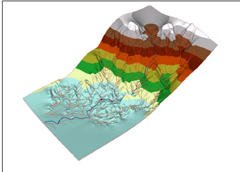
Figure 8. Screenshot of a 3-dimension model of the watershed of Rio Espíritu Santo using ArcScene. Blue line is the river, black dot is USGS water gage station, red lines are streams and tributaries. Vertical exaggregation is 5X.
