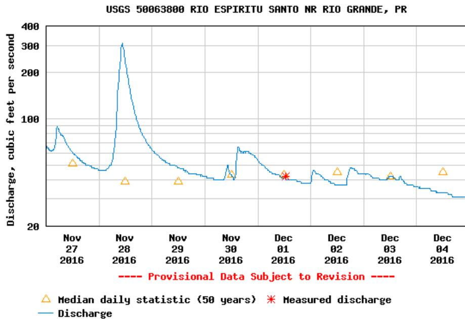
Figure 7. Graphic showing the weekly discharge of Rio Espíritu Santo (blue line), high peak shows high discharge produced by a precipitation event, triangles are median daily statistics during 50 years and red asterisk field measurement.
