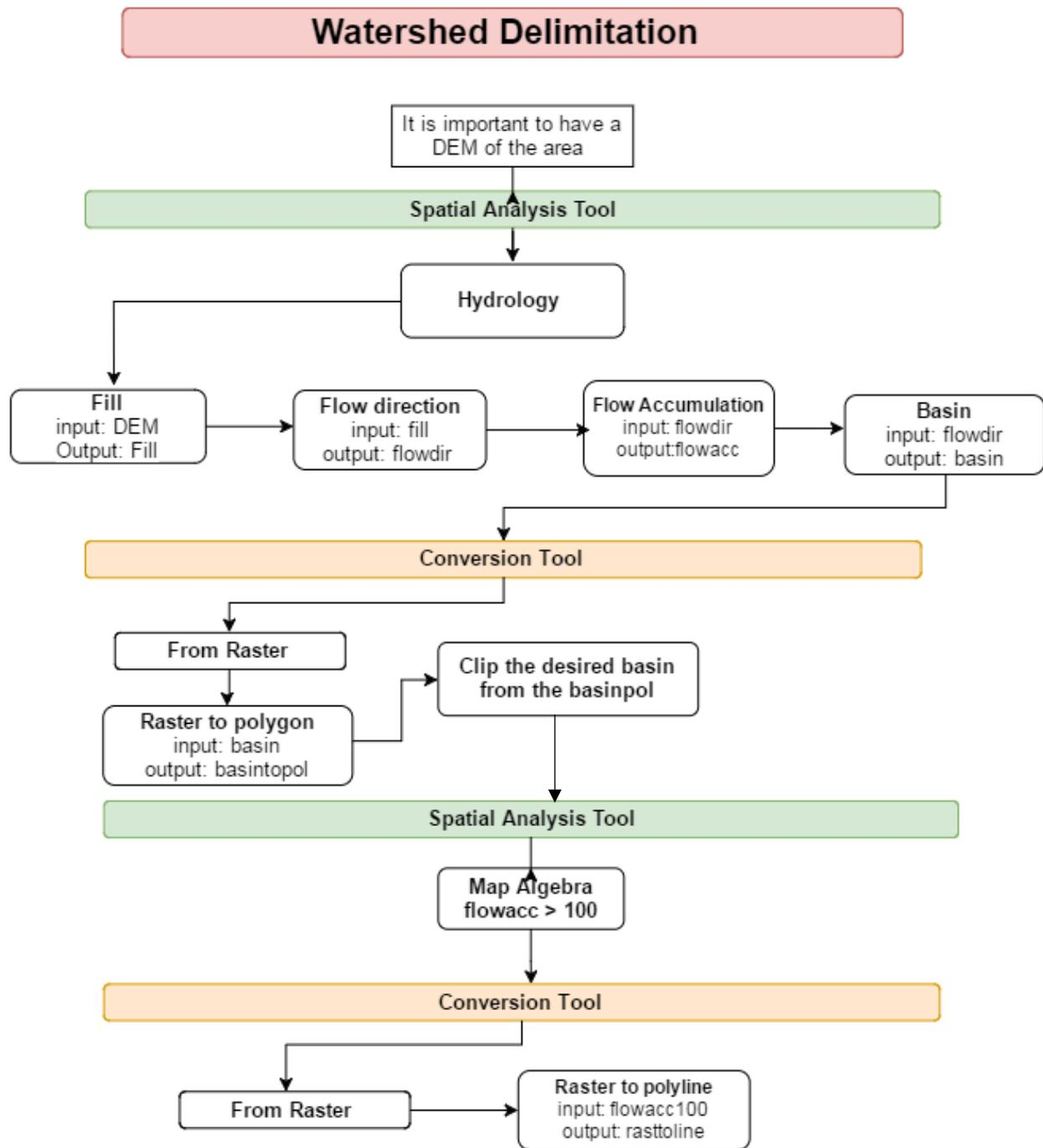
Figure 1. Flowchart showing how to delineate a watershed using ArcMap. A digital elevation model (DEM) file is needed to start the process.
