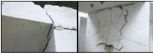
Figure 12. Failure mechanisms of the first two specimens tested: (a) joint failure of specimen 1 (without concrete block wall), (b) concrete wall failure of specimen 2 (with concrete block wall).
