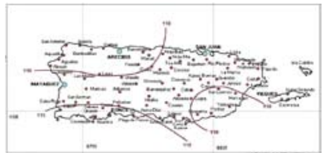
Figure 9: Contours of maximum wind speed for 100 year return period.
