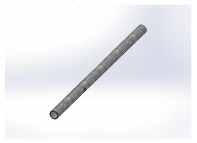
This part features a shorter length due to the elbow connectors being larger than anticipated.
