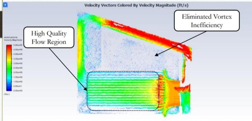
**Figure 9:** Final kiln design center plane velocity vector field.
