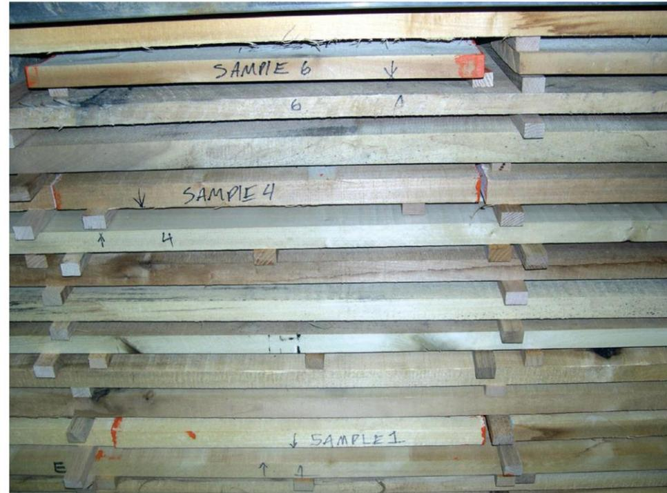
Figure 9—Pack of lumber with sample boards.
