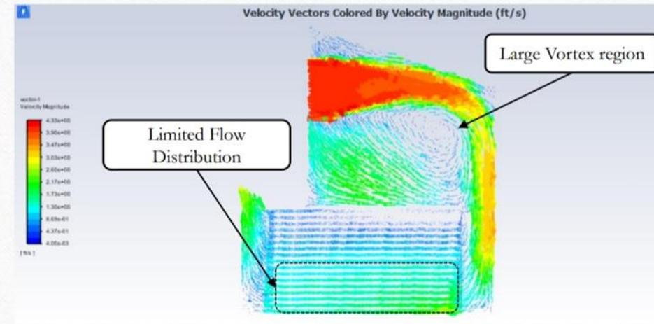
**Figure 10:** Initial kiln design center plane velocity vector field.
