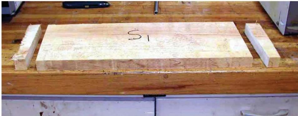
Figure 7—Dimensions and picture of sample board for controlling the drying process.
