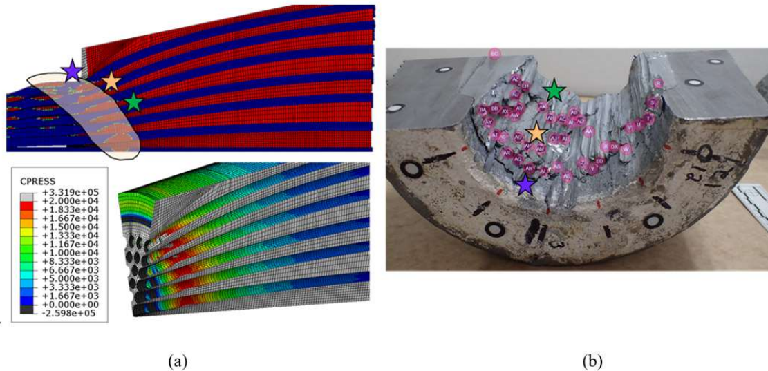
Figure 8: Stress distribution and failure mode: (a) highest stresses were not predicted to be planar; (b) failure surface followed a spheroid shape, matching stepped patterns seen in forensic evidence.
