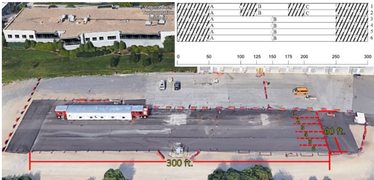
Figure 4: Dimensions of pavement test sections.
