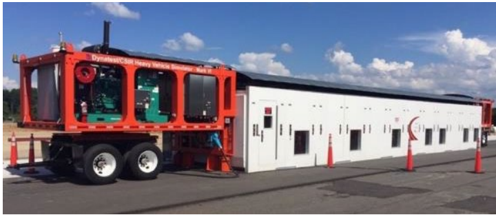
Figure 2: HVS MK VI testing on Lane 4, Cell A.
