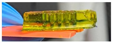
The latest prototype consists of a  $4 \times 5$  array of chambers for high-throughput organoid growth, along with inlet/outlet for perfusion flow of nutrients to avoid necrosis. The device is  $20 \times 10 \times 5$  mm with both channels and chambers of 1.0 mm diameter.
