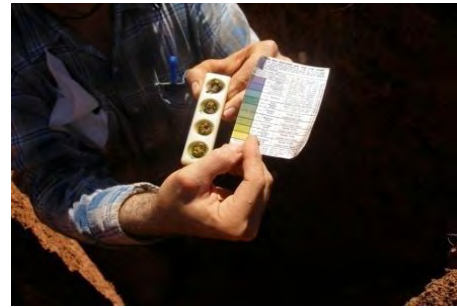
Figure 3.1 Field pH Determination Using the Hellige-Truog Soil Reaction Tester
