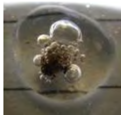
Figure 3.2 Effervescent reaction during manganese features test
